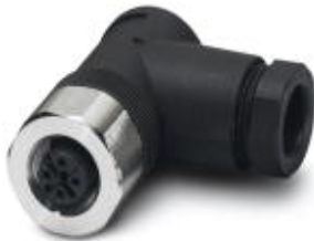
Sensor/actuator connector, female, angled, 5-pos., M12, screw connection, high-grade steel knurl, cable screw connection Pg9
