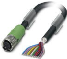
Sensor/Actuator cable, 12-position, PUR/PVC, Black RAL 9005, shielded, Free cable end, on Socket straight M12 SPEEDCON, A-coded, Cable length: 10 m
