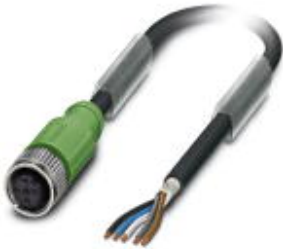
Sensor/Actuator cable, 5-position, PUR halogen-free, Black-gray RAL 7021, shielded, Free cable end, on Socket straight M12, A-coded, Cable length: 1.5 m
