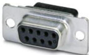
D-SUB contact carrier, shell size 1, for nine signal contacts, contact type socket, for crimp contacts, straight, fixing with a 3 mm hole, for panel mounting frame and sleeve housing VS-09-...
