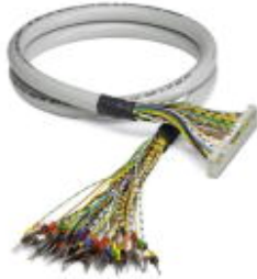
Round cable assembled with a 14-pos. socket strip and an open end. On the open end, the wires are labeled with 1 to 14 and have ferrules, cable length: 1 m
