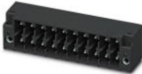
Header, Nominal current: 8 A, Rated voltage (III/2): 160 V, Number of positions: 5, Pitch: 3.5 mm, Color: Black, Contact surface: Tin, Assembly: SMD/THT/THR
