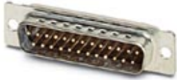
D-SUB contact insert, shell size 3, with 25 signal contacts, contact type pin, with solder cup, straight, fixing with a 3 mm hole, for panel mounting frame and sleeve housing VS-25-...
