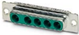
D-SUB contact carrier, shell size 3, accommodation for five combined contacts, contact type socket, straight, fixing with a 3 mm hole, for panel mounting frame and sleeve housing VS-25-...
