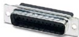
D-SUB contact carrier, shell size 3, for 25 signal contacts, contact type pin, for crimp contacts, straight, fixing with a 3 mm hole, for panel mounting frame and sleeve housing VS-25-...
