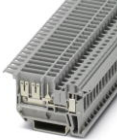
Feed-through terminal block, Connection type: Screw connection, Slip-on connection, Cross section: 0.2 mm 2 - 4 mm 2 , AWG :20- 14, Width: 6.2 mm, Color: gray, Mounting: NS 35/7,5, NS 35/15
