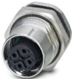
Sensor/actuator flush-type socket, 5-pos., M12-SPEEDCON, shielded, B-coded, rear/screw mounting with Pg9 thread, with straight solder connection
