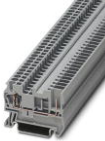
Feed-through terminal block, Connection method: Spring-cage/plug-in connection, Cross section: 0.08 mm 2 - 4 mm 2 , AWG: 28 - 12, Width: 5.2 mm, Color: gray, Mounting type: NS 35/7,5, NS 35/15
