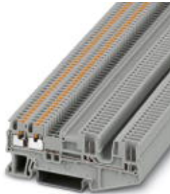
Feed-through terminal block, Connection method: Push-in / plug connection, Cross section: 0.14 mm 2 - 1.5 mm 2 , AWG: 26 - 14, Width: 3.5 mm, Color: gray, Mounting type: NS 35/7,5, NS 35/15
