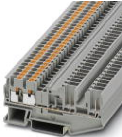
Feed-through terminal block, Connection method: Push-in / plug connection, Cross section: 0.14 mm 2 - 4 mm 2 , AWG: 26 - 12, Width: 5.2 mm, Color: gray, Mounting type: NS 35/7,5, NS 35/15
