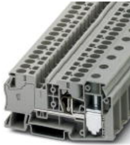
Feed-through terminal block, Connection method: Screw connection, Cross section: 1.5 mm 2 - 50 mm 2 , AWG: 16 - 1/0, Width: 16.2 mm, Color: blue, Mounting type: NS 35/7,5, NS 35/15
