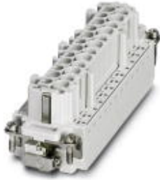
HEAVYCON female insert, B24 series, 24-pos., for crimp contacts. PE connection using tension sleeve technology.
