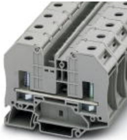
Feed-through terminal block with bolt connection, cross section: 2.5 - 35 mm 2 , AWG: 14 - 2, width 20.2 mm, color: Gray
