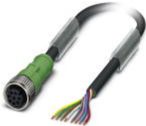
Sensor/Actuator cable, 8-position, PUR halogen-free, Black-gray RAL 7021, Free cable end, on Socket straight M12, A-coded, Cable length: 5 m
