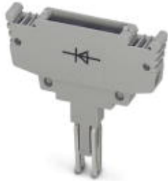
Component plug, with universal diode, to connect 2-pos. components into the basic terminal block, height: 19 mm, color: Gray
