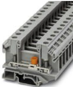
Universal terminal block with bolt connection, with test socket screws and disconnect slide, cross section: 0.1 - 6 mm 2 , width: 11 mm, color: Gray
