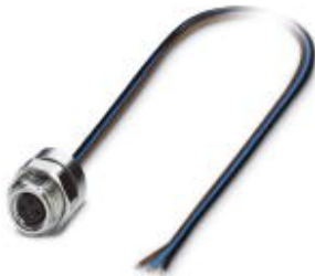
Sensor/actuator flush-type socket, 3-pos., M8, rear/screw mounting, with M12 thread, with 0.5 m TPE litz wire, 3 x 0.25 mm 2
