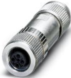
Bus system connector, PROFINET CAT5, PROFINET CAT5e, 4-position, shielded, Socket straight M12, D-coded, Insulation displacement connection, Knurl material: Nickel-plated brass, External cable diameter 4 mm ... 8 mm
