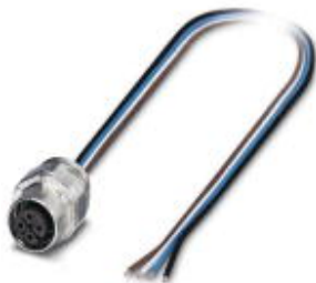
Sensor/actuator flush-type socket, 4-pos., M12 SPEEDCON, A-coded, front/screw mounting with M16 thread, can be positioned, with 0.5 m TPE litz wire, 4 x 0.34 mm 2
