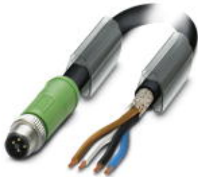
Sensor/Actuator cable, 4-position, PUR halogen-free, Black RAL 9005, shielded, Plug straight M12 SPEEDCON, T-coded, on Free cable end, Cable length: 5 m
