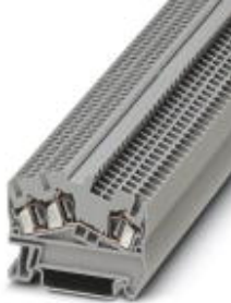
Feed-through terminal block, Connection method: Spring-cage connection, Cross section: 0.08 mm 2 - 4 mm 2 , AWG: 28 - 12, Width: 5.2 mm, Color: gray, Mounting type: NS 35/7,5, NS 35/15
