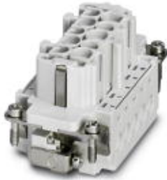
HEAVYCON female insert, B10 series, 10-pos., screw connection. PE connection using tension sleeve technology.
