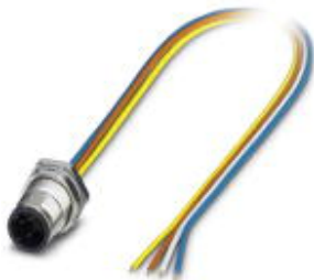
Bus system flush-type plug, 4-pos., M12 SPEEDCON, D-coded, front/screw mounting with M12 thread, with 0.5 m TPE litz wire, 4 x 0.34 mm 2
