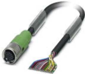
Sensor/Actuator cable, 17-position, PVC, Black RAL 9005, Free cable end, on Socket straight M12 SPEEDCON, A-coded, Cable length: 10 m
