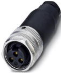
Sensor/actuator connector, female, straight, 3-pos., 7-8", screw connection, metal knurl, cable screw connection Pg9
