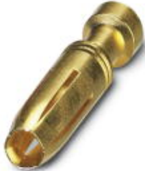
Turned 2.5 crimp contact, individual female contact, core diameter 1.5 mm 2 , gold-plated
