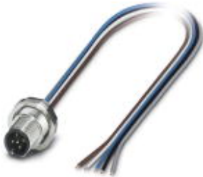
Sensor/Actuator flush-type plug, 5-pos., M12, A-coded, rear/screw mounting with Pg9 thread, with 0.5 m TPE litz wire, 5x 0.34 mm 2
