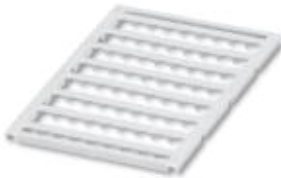
Terminal marking, Sheet, white, Unlabeled, Can be labeled with: BLUEMARK CLED, BLUEMARK LED, Plotter, Mounting type: Plug in, For terminal block width: 7.5 mm, Lettering field: 3.97 x 6.9 mm
