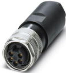
Sensor/actuator connector, female, straight, 5-pos., 7-8", screw connection, metal knurl, Pg11 cable gland
