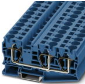
Feed-through terminal block, Connection method: Spring-cage connection, Cross section: 0.2 mm 2 - 25 mm 2 , AWG: 24 - 4, Width: 12.2 mm, Color: blue, Mounting type: NS 35/15, NS 35/7,5
