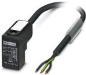
Sensor/Actuator cable, 3-position, PUR halogen-free, Black-gray RAL 7021, Free cable end, on Valve connector CI (9.4 mm), with 1 LED, connected with Z diode, Cable length: 3 m
