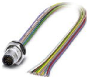
Sensor/actuator flush-type plug, 17-pos., M12 SPEEDCON, rear/screw mounting with M16 thread, with 0.5 m halogen-free TPE litz wire, 17 x 0.14 mm²
