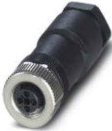
Connector, Universal, 4-position, Socket straight M12, T-coded, Screw connection, Knurl material: Zinc die-cast, nickel-plated, Cable gland Pg11, External cable diameter 8 mm ... 10 mm
