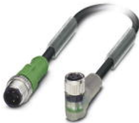
Sensor/Actuator cable, 3-position, PUR halogen-free, Black-gray RAL 7021, Plug straight M12, A-coded, on Socket angled M8, with 2 LEDs, Cable length: 1.5 m
