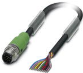
Sensor/Actuator cable, 12-position, PVC, Black RAL 9005, Plug straight M12 SPEEDCON, A-coded, on Free cable end, Cable length: 10 m
