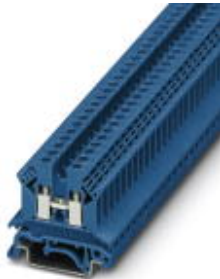
Feed-through terminal block, Connection method: Screw connection, Cross section: 0.2 mm 2 - 4 mm 2 , AWG: 24 - 12, Width: 6.2 mm, Color: blue, Mounting type: NS 35/7,5, NS 35/15
