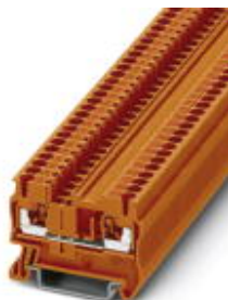
Feed-through modular terminal block, connection method: Push-in, cross section: 0.08 mm 2 - 4 mm 2 , AWG 28 - 12, width: 5.2 mm, color: orange, mounting: NS 35/7.5, NS 35/15
