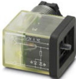
Valve connector, 3-pos., construction BI, 1 LED, with protective circuit, screw connection, M16 cable gland
