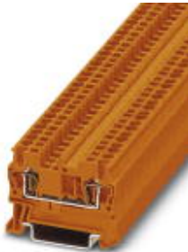
Feed-through terminal block, Connection method: Spring-cage connection, Cross section: 0.08 mm 2 - 4 mm 2 , AWG: 28 - 12, Width: 5.2 mm, Color: orange, Mounting type: NS 35/7,5, NS 35/15
