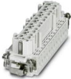
HEAVYCON female insert, B24 series, 24-pos., 25 ... 48 color print, screw connection. PE connection using tension sleeve technology.
