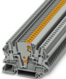
Test disconnect terminal block, Connection method: Screw connection with test socket screws, Cross section: 0.14 mm 2 - 6 mm 2 , AWG: 26 - 10, Width: 6.2 mm, Color: gray, Mounting type: NS 35/7,5, NS 35/15
