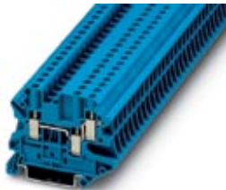
Feed-through terminal block, Connection method: Screw connection, Cross section: 0.14 mm 2 - 6 mm 2 , AWG: 26 - 10, Width: 6.2 mm, Color: blue, Mounting type: NS 35/7,5, NS 35/15
