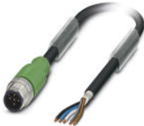
Sensor/Actuator cable, 5-position, PUR halogen-free, Black-gray RAL 7021, shielded, Plug straight M12, A-coded, on Free cable end, Cable length: 10 m
