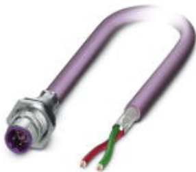
Bus system flush-type plug, PROFIBUS, 2-pos., M12, shielded, B-coded, SPEEDCON, rear/screw mounting with Pg9 thread, with 2.0 m bus cable, 2 x 0.25 mm 2
