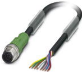
Sensor/Actuator cable, 8-position, PUR halogen-free, Black-gray RAL 7021, Plug straight M12, A-coded, on Free cable end, Cable length: 5 m
