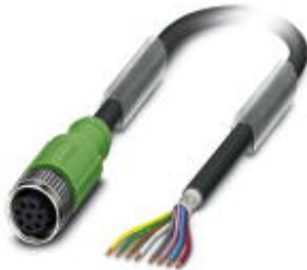
Sensor/Actuator cable, 8-position, PUR halogen-free, Black-gray RAL 7021, shielded, Free cable end, on Socket straight M12, A-coded, Cable length: 5 m
